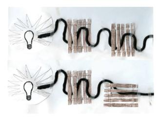
the drawings where the fence represents the filter and the wavy line is a light ray. In the first drawing, a light wave that is on the same plane as the gap of the picket fence can make it through. Light waves that do not line up with the gap are blocked. When it comes to a fence that has the same orientation, the light wave continues. If the second fence is at right angles, the light wave is blocked and only a small amount of light gets through.
