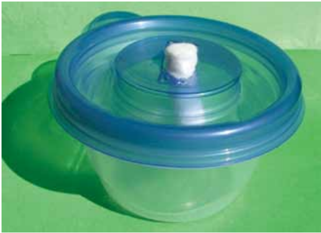
Figure 5.9 A simple nectar feeder consisting of a dental wick and plastic container. The feeder is placed below the starter box with the wick protruding through the floor.
