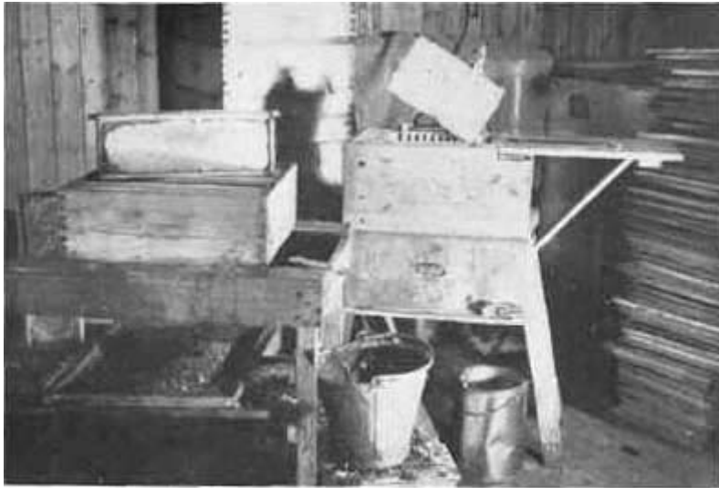
20. Heather honey press, Raynor type, as used by us
