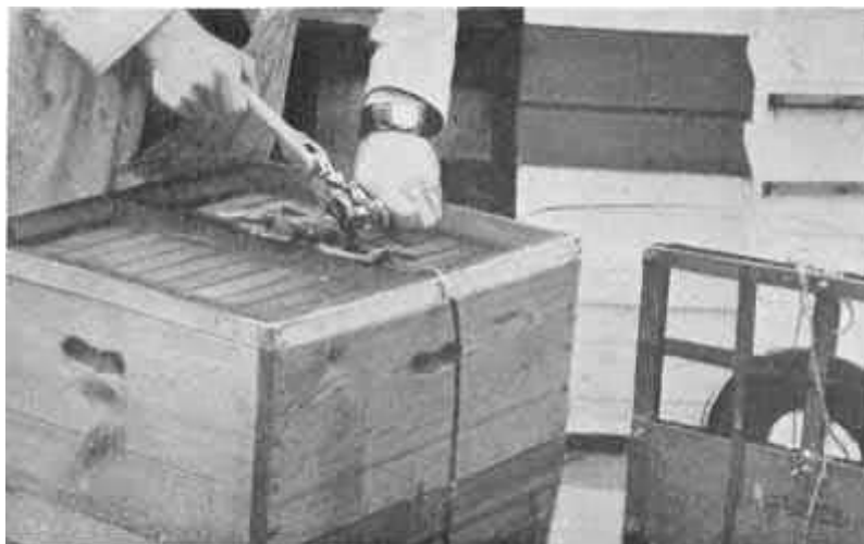
16. Using a 'Signode' strapping machine on a screened hive
