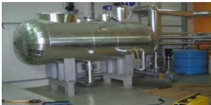
Photo 3. Melting and resting tanks for beeswax
