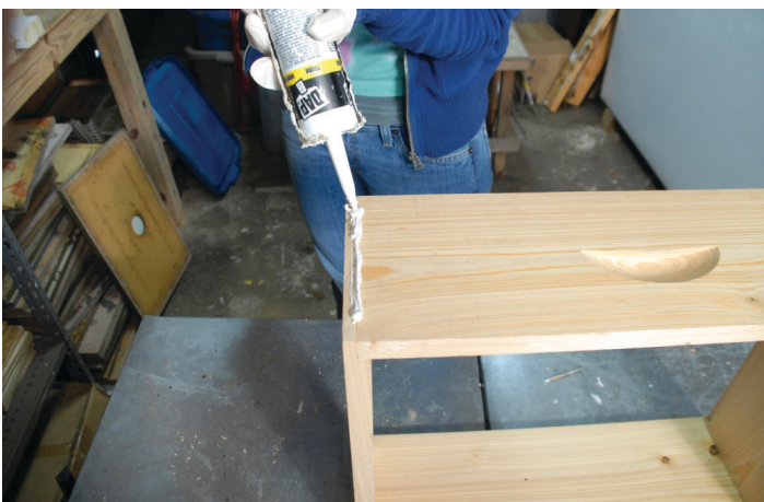
Figure 3. Caulking joints helps seal out moisture.
