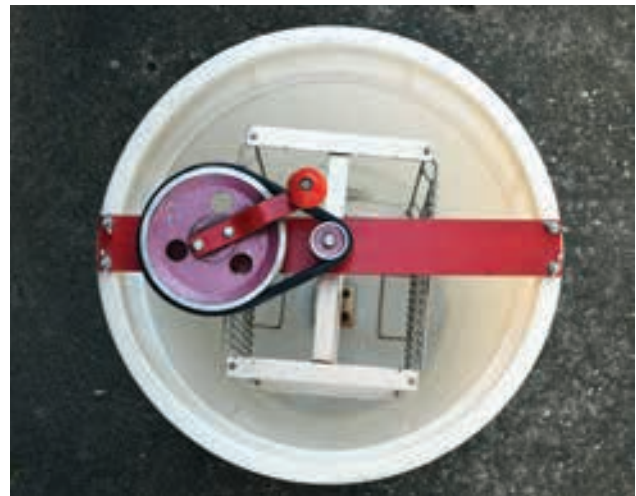
Interior view of 2-frame polygenic extractor.
