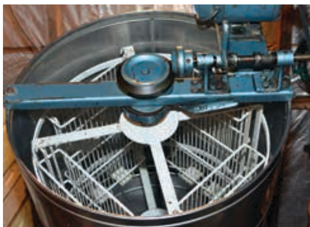
Interior view of the 4-frame extractor. The hinged baskets allow the combs to be turned (reversed) for extracting the second side of the comb. Note that the cover and safety guards provided by the manufacturer have been temporarily removed for this photo to be taken.
