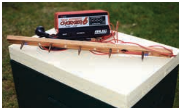
Electric embedder and 6-volt power source.
