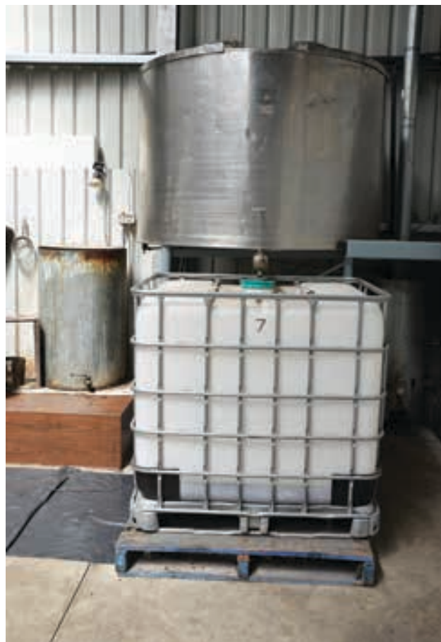
A stainless steel settling tank (top) and intermediate bulk container.
