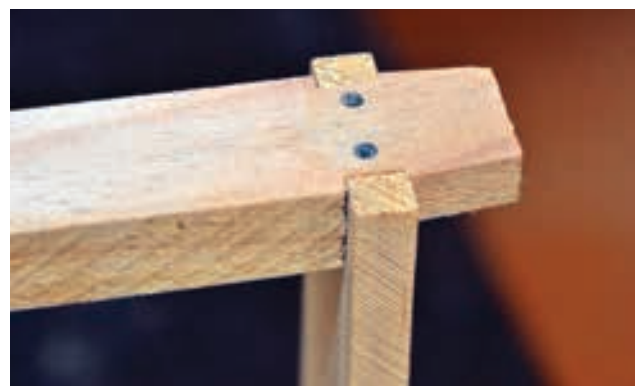
Nail the top bar next using two nails.
