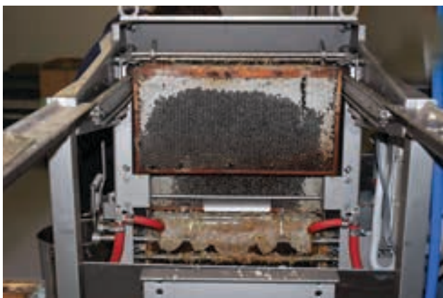
The feed-in end of an uncapping machine showing the cutting blades.
