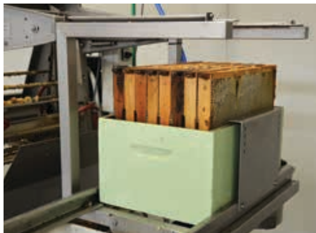
An uncapping machine. On the bottom right hand side of the photo an operator (not in view) uses a paint scraper to remove burr comb from the top bars of the uncapped frames and combs. The uncapped combs appear on the rack at the bottom of the photo.
