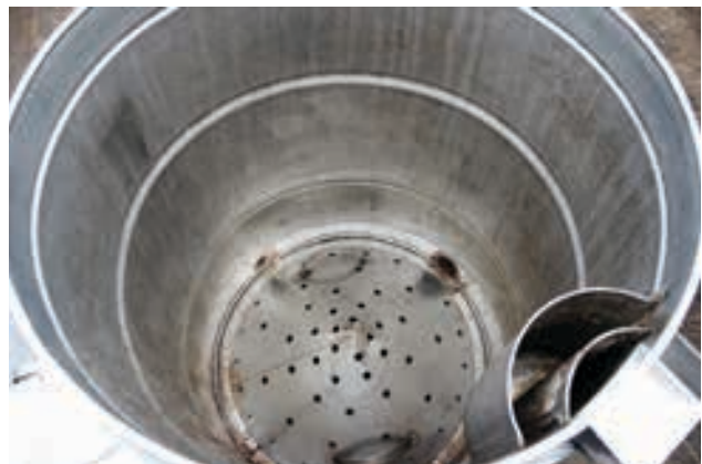
The inside of an electric melter.
