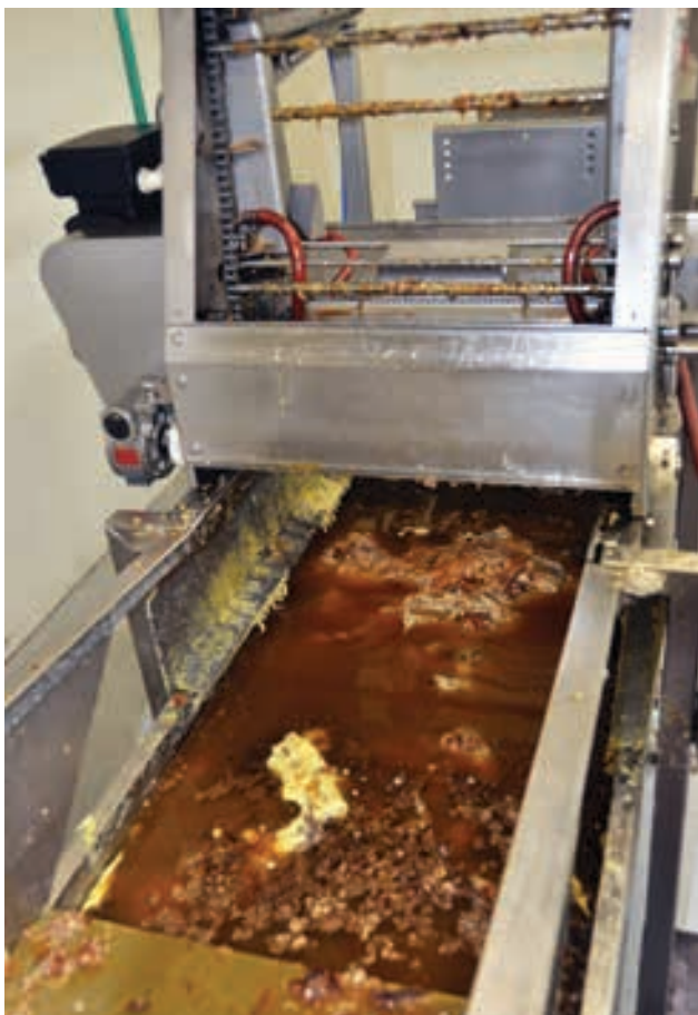
A commercial wax reducer positioned below an uncapping machine.
