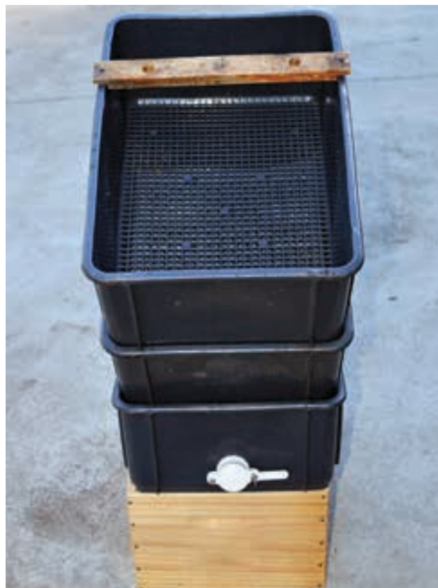
Polygenic uncapping unit showing coarse mesh. The frame to be uncapped is placed on the upward projecting spike positioned at the centre of the timber support.
