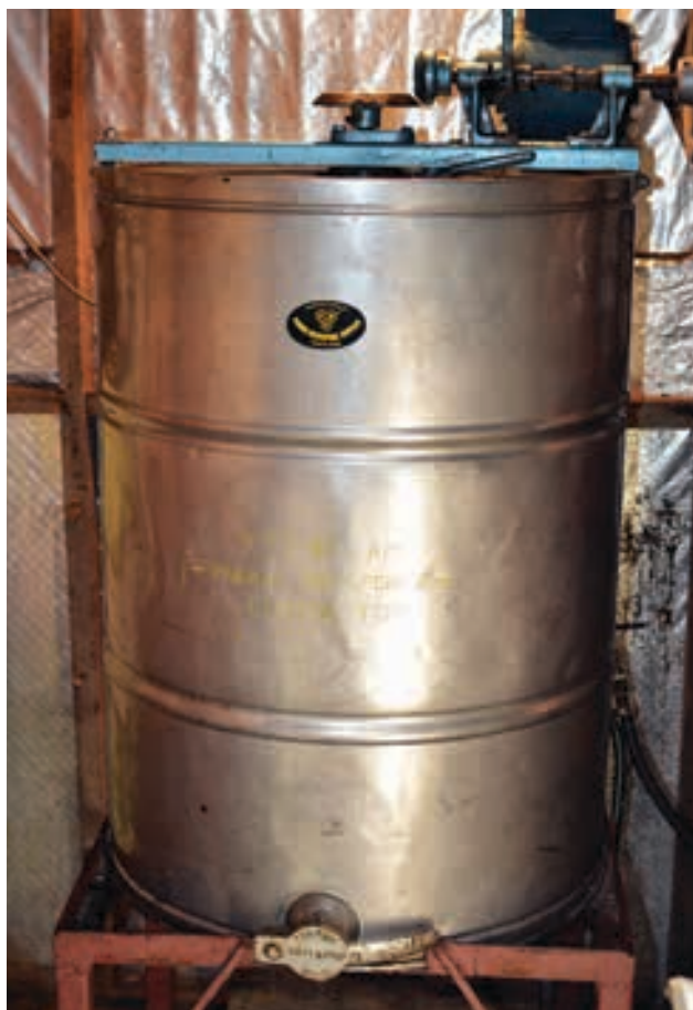
A 4-frame, stainless steel, electric driven extractor on stand.
