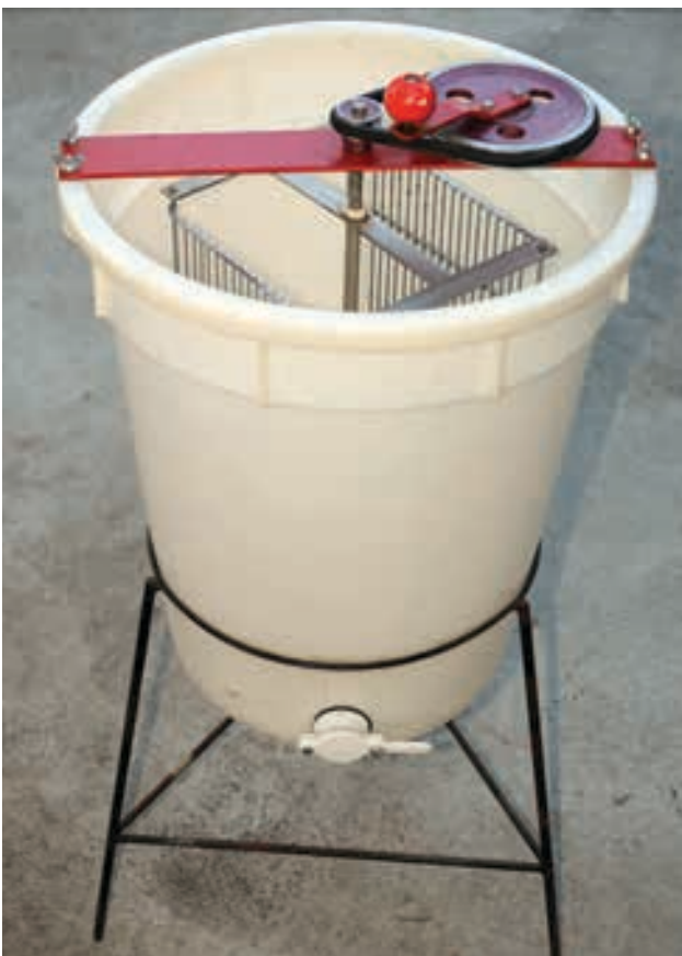
Hand operated 2-frame polygenic extractor on stand.
