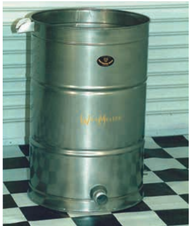
A commercially available beeswax melter suitable for cappings and burr comb.
