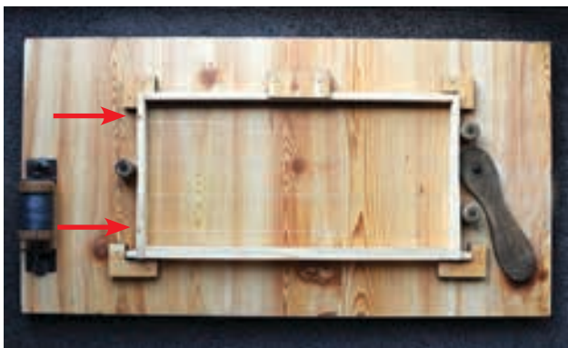
Homemade wiring board with wired frame. Note the position of the two gimp tacks on the left end bar indicated by the arrows.
