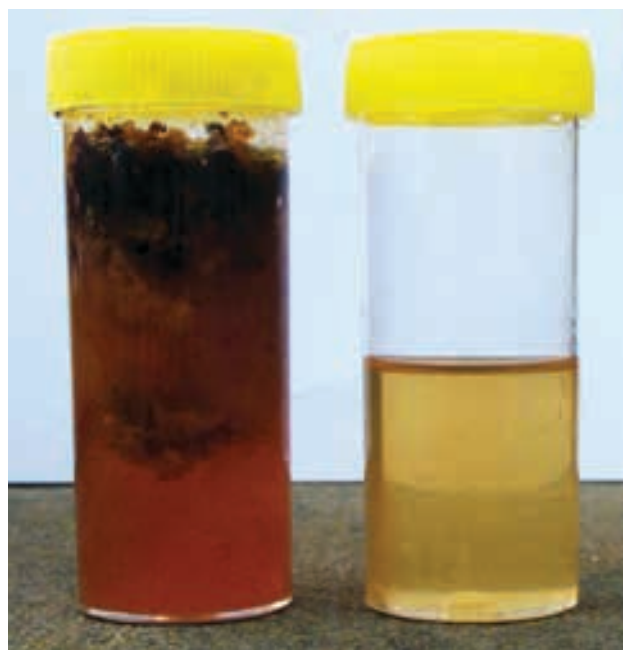
These samples of honey are unsuitable for testing. Left, the honey must not contain dirt and wax; right, the container must be filled with honey.
